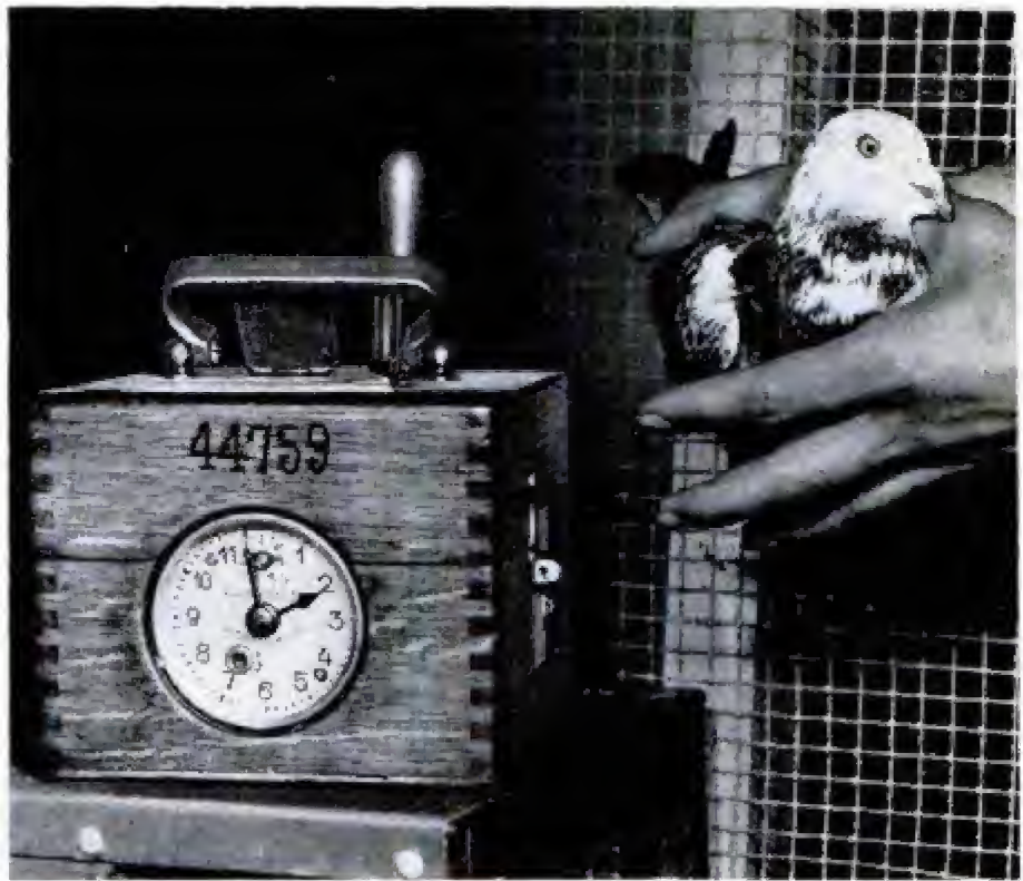
Each owner gets a sealed clock before the race. When his bird returns, he removes band from its leg, drops it in clock which registers the time
